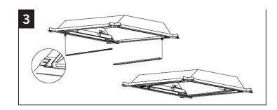
4. Using the included self-tapping screws, use electronic screwdriver to secure brackets into place through bracket mounting holes from inside of the fixture. Caution: Luminaire wiring and electrical parts may be damaged when drilling for installation of LED retrofit kit. Ensure that enclosed wiring and components have not been damaged.
