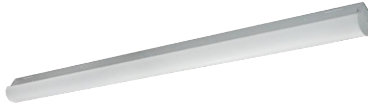
8' LED Microstrip Fixture, 120–277V Input, Frosted Lens, 0–10V Dimming
